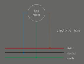
Please note: electrical pull of the awning motor is less than 3A
